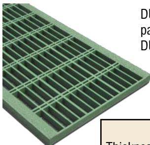
DURAGRATE® molded fiberglass stair treads are available in a 1-1/2" thick 1-1/2" x 6" rectangular mesh pattern. The standard panel size is 22-1/2" x 10'. Stair treads can be produced in any of the standard DURAGRATE® resin systems. The stair tread panel comes complete with anti-slip nosing.
